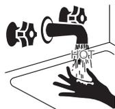
Hot Water Heater temperature over 125 °F can cause severe burns instantly or death from scalding.
